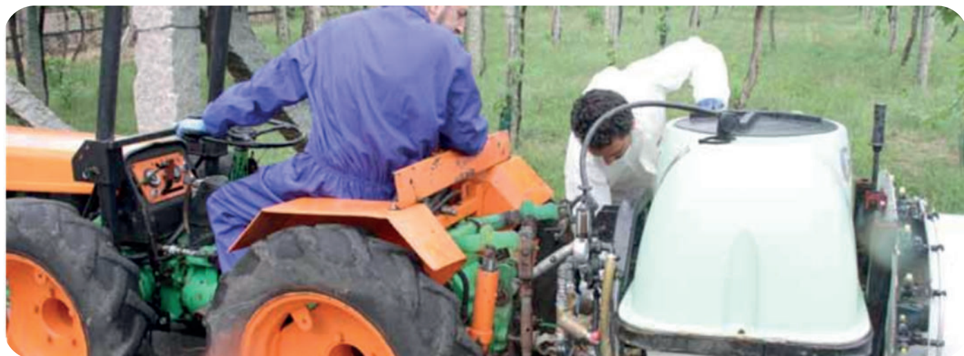
Place the implements on flat, firm surfaces with appropriate brackets and slowly bring the tractor as close to them as you can.
