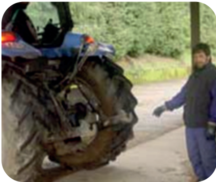
No one should put their hands near the hitch area when the tractor is moving.
