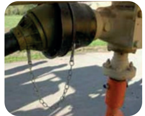
Report any failure or deterioration of the transmission shaft protections.
