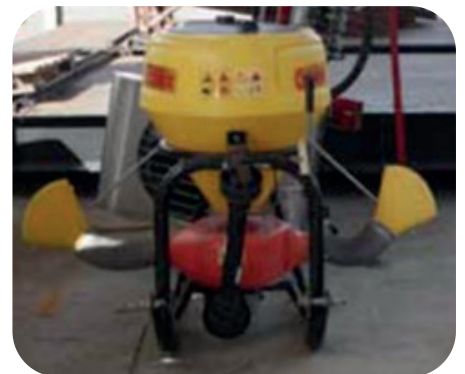
The implement must be well stabilized, with good supports adapted to the equipment, stable, firm, and resistant. Only use supports specifically manufactured to secure the implement.
