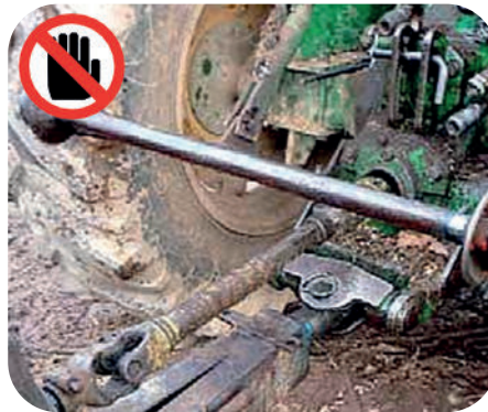
Report any failure or deterioration of the transmission shaft protections.
