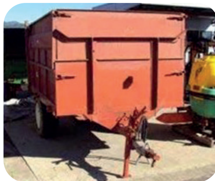
The implement must be well stabilized, with good supports adapted to the equipment, stable, firm, and resistant. Only use supports specifically manufactured to secure the implement.
