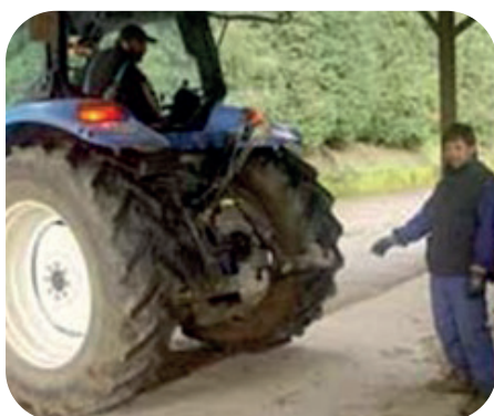
Place the implements on flat, firm surfaces with appropriate brackets and slowly bring the tractor as close to them as you can.
