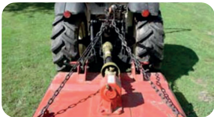
Make sure you have the right implement for the power and weight of the tractor.
