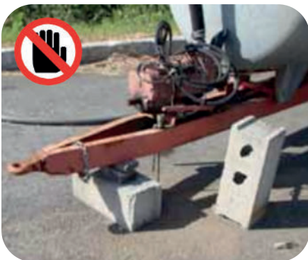
The implement must be well stabilized, with good supports adapted to the equipment, stable, firm, and resistant. Only use supports specifically manufactured to secure the implement.
