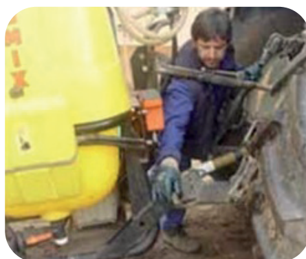
If there is a person between the implement and the tractor, do not engage reverse gear.
