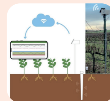
Fig. 4. Soil moisture content monitoring systems associated with new technologies (adapted from Tomaz et al., 2022).
